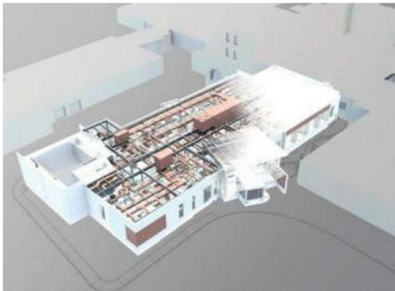
*The new Marlborough (Mass.) Hospital Cancer Pavilion is connected to the existing hospital by a CMU shear wall that contains grouted cells and bond beams that are impermeable. This situation left minimal space for 12 individual services to pass from the hospital to the new wing. The key trades met over a 12-week period to find a workaround and untangle the limited space above the ceiling.*
